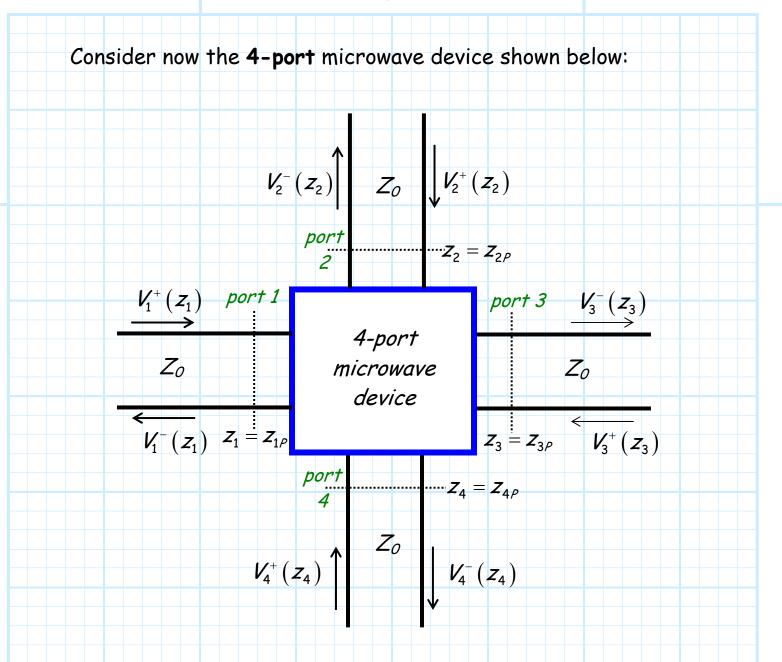
Note that we have now characterized transmission line activity in terms of incident and "reflected" waves. Note the negative going "reflected" waves can be viewed as the waves **exiting** the multi-port network or device.
