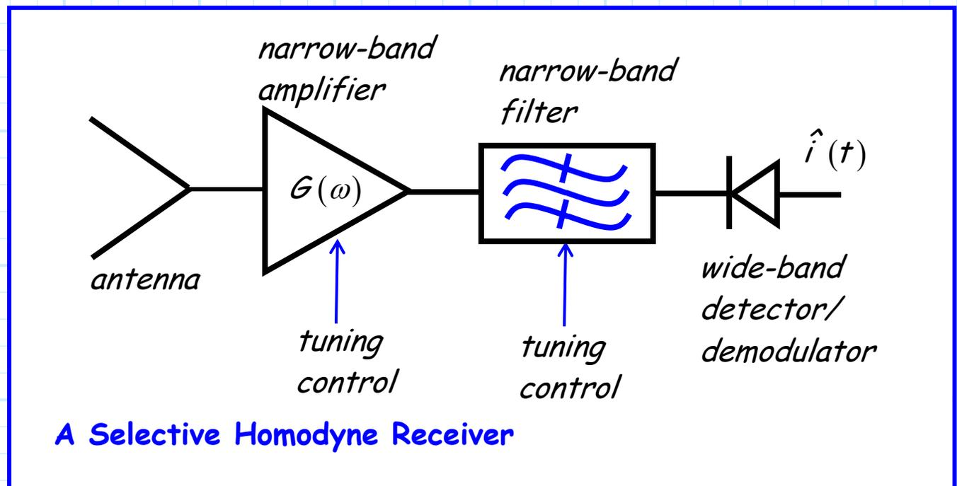
Therefore, if we tune **both** the amplifier and filter to frequency  $\omega_4$ , we might get:
