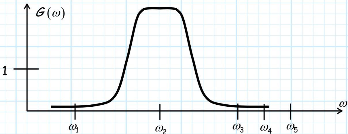
Therefore, the gain in the pass-band is **large** ( $G(\omega) \gg 1$ ), while **outside** the pass-band the gain is **small** ( $G(\omega) \ll 1$ ).
