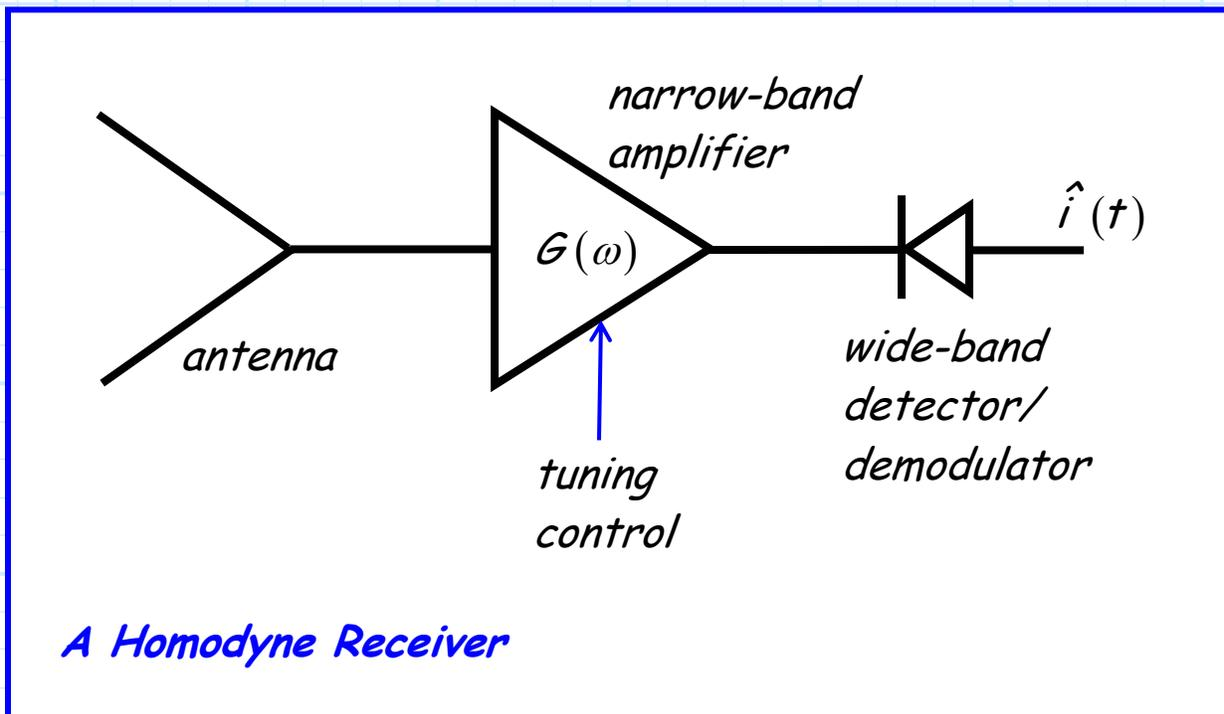
The **desired** radio signal was selected by **tuning** a narrow-band amplifier!
