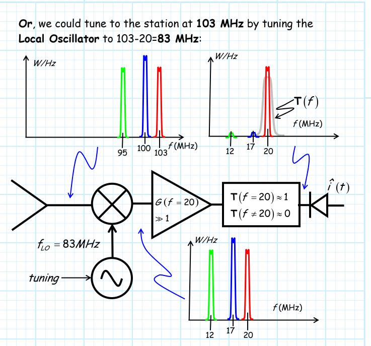
**Q:** Wait a second! You mean we need to **tune** an oscillator. How is that any **better** than having to **tune** an amplifier and/or filter?
