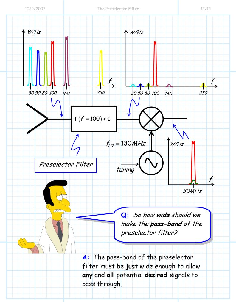
\* Consider our example of  $f_s$  = 100 MHz. This signal is smack-dab in the middle of the FM radio band, and so let's assume it is an FM radio station (if it were, it would actually be at frequency 100.1 or 99.9 MHz).
