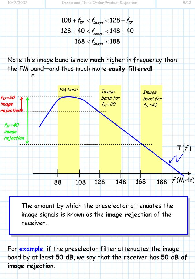
So by **increasing** the receiver IF frequency, we can **either** get greater image rejection from the same preselector filter order, **or** we can reduce the preselector filter order while maintaining sufficient image rejection.
