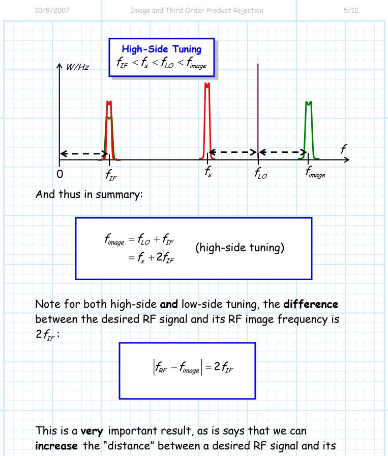
image frequency by simply **increasing** the IF frequency of our **receiver design**!
