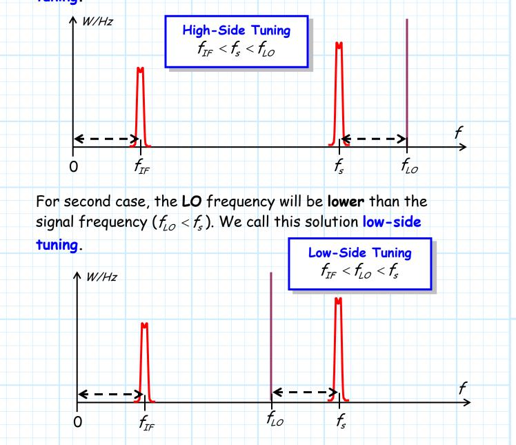
For example, consider again the FM band. Say a radio engineer is designing an FM radio, and has selected an IF frequency of 30 MHz. Since the FM band extends from 88 MHz to 108 MHz (i.e., 88 MHz  $\leq f_s \leq 108$  MHz), the radio engineer has two choices for LO bandwidth.
