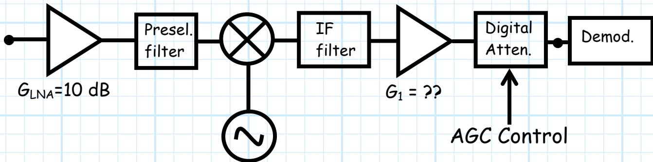
The designer of this receiver has yet to select the **fixed** gain  $G_1$  of an **amplifier** in the IF section. For this design, there is actually a **range** of fixed amplifier gain values that will work (i.e., allow **any** signal within the receiver dynamic range to be accurately demodulated).
