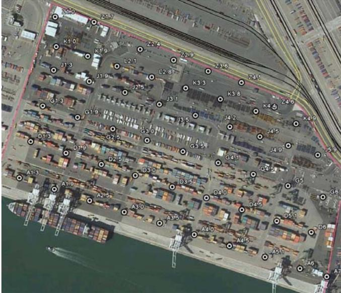
**Figure 8 Oakland International Container Terminal light pole locations**
