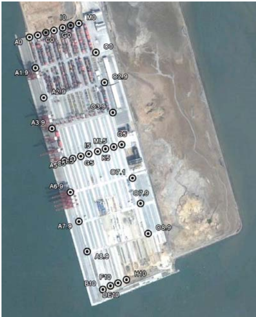
Figure 9 Da Chan Bay Terminal rectangle boundary light pole pattern
