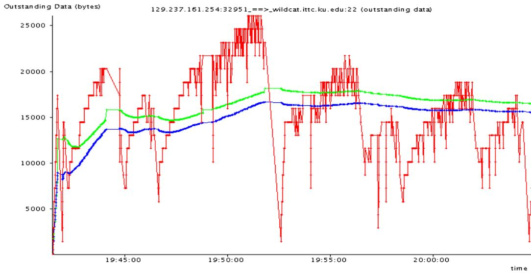
**Figure 5.21 Outstanding unacknowledged data of a video upload**
