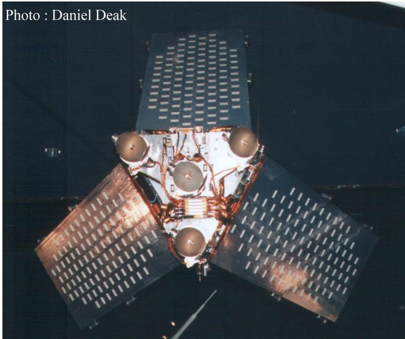
**Figure 2.6: The three panels of an Iridium phased array antenna (Source: [12])**
