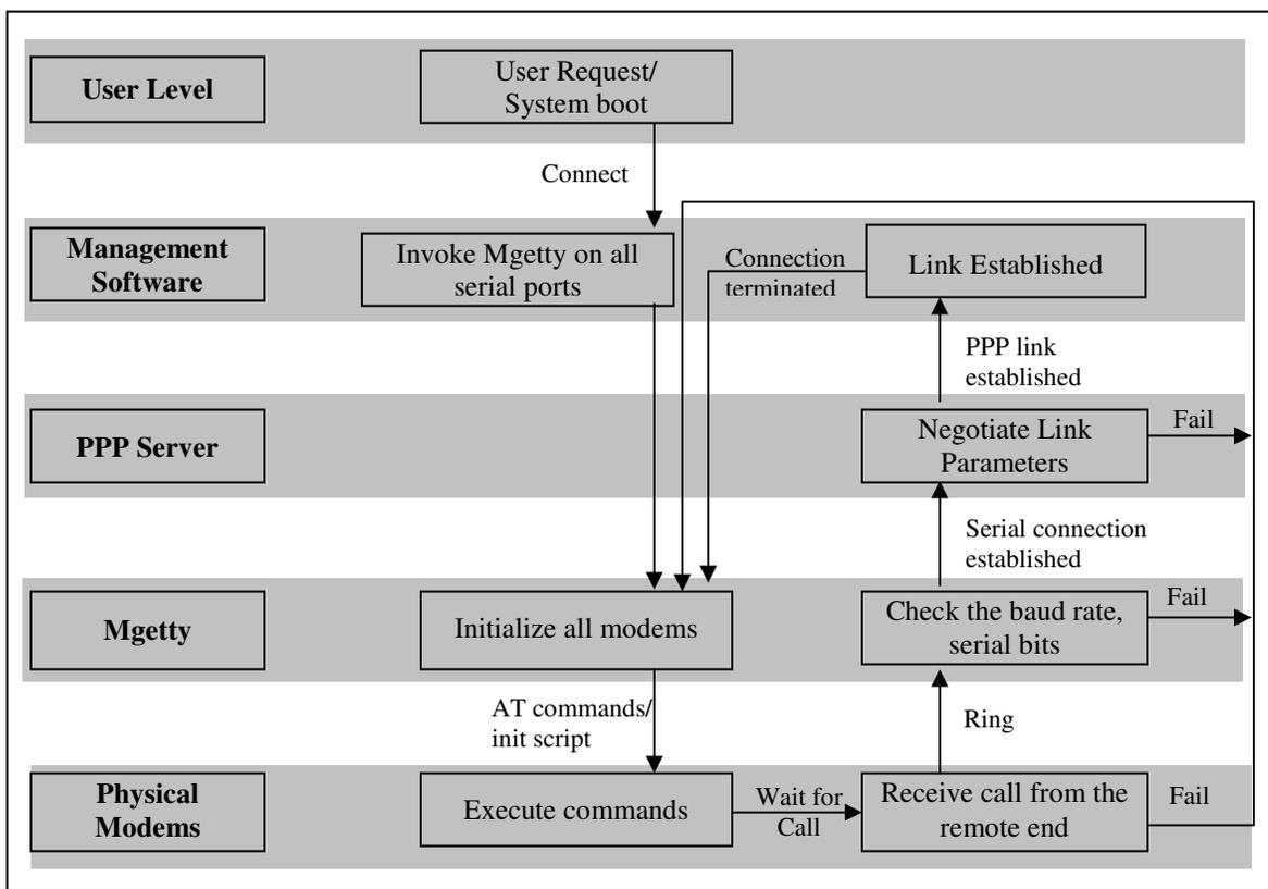
**Figure 4.4 Software flow control of the local system (server)**
