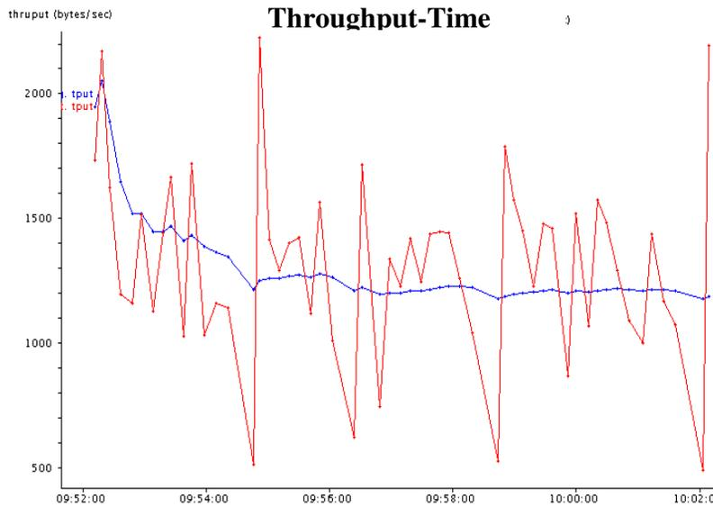
Figure 5.34 Throughput of the mobile 4-channel system during second test
