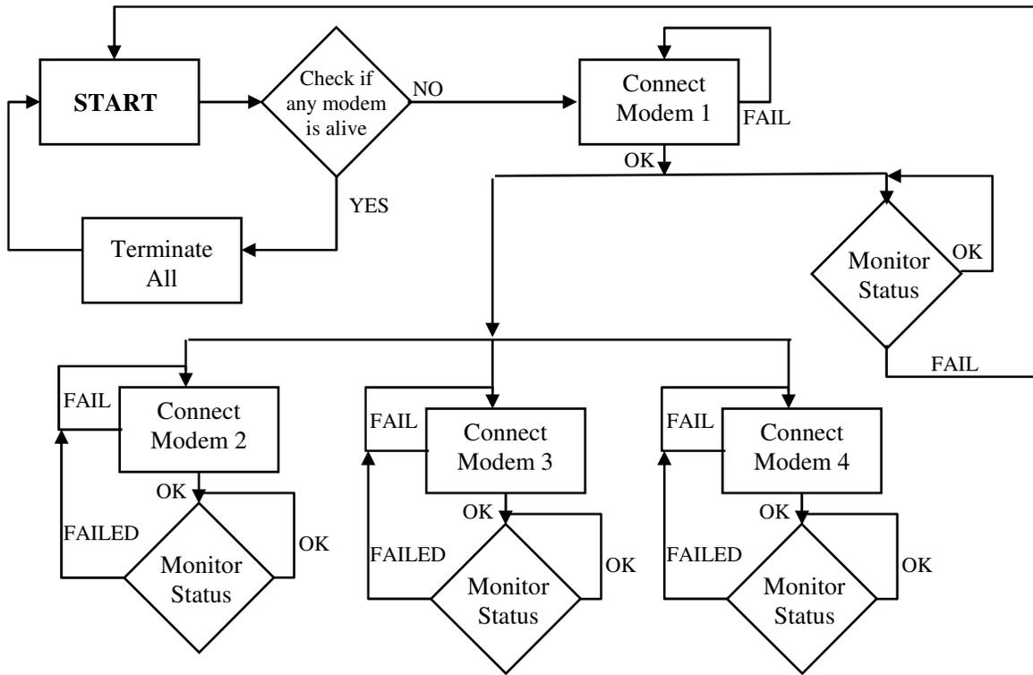
**Figure 4.5 Modem flow control diagram**
