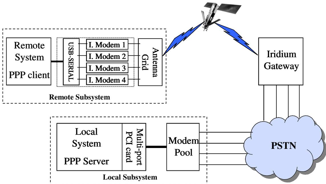
Figure 4.1 Four-channel Iridium communication system
