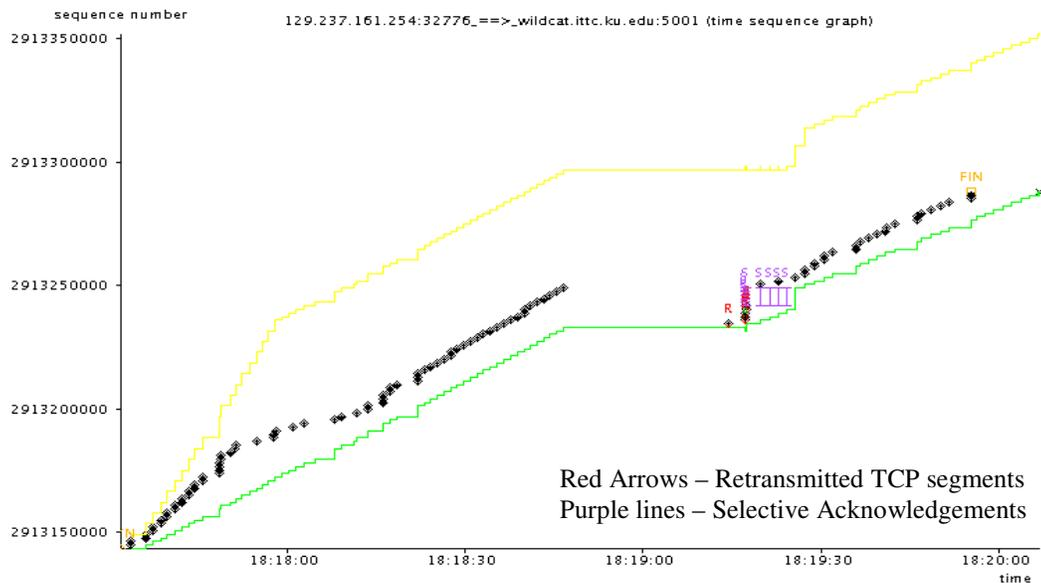
**Figure 5.28 Time sequence graph of a TCP connection with a single link termination**
