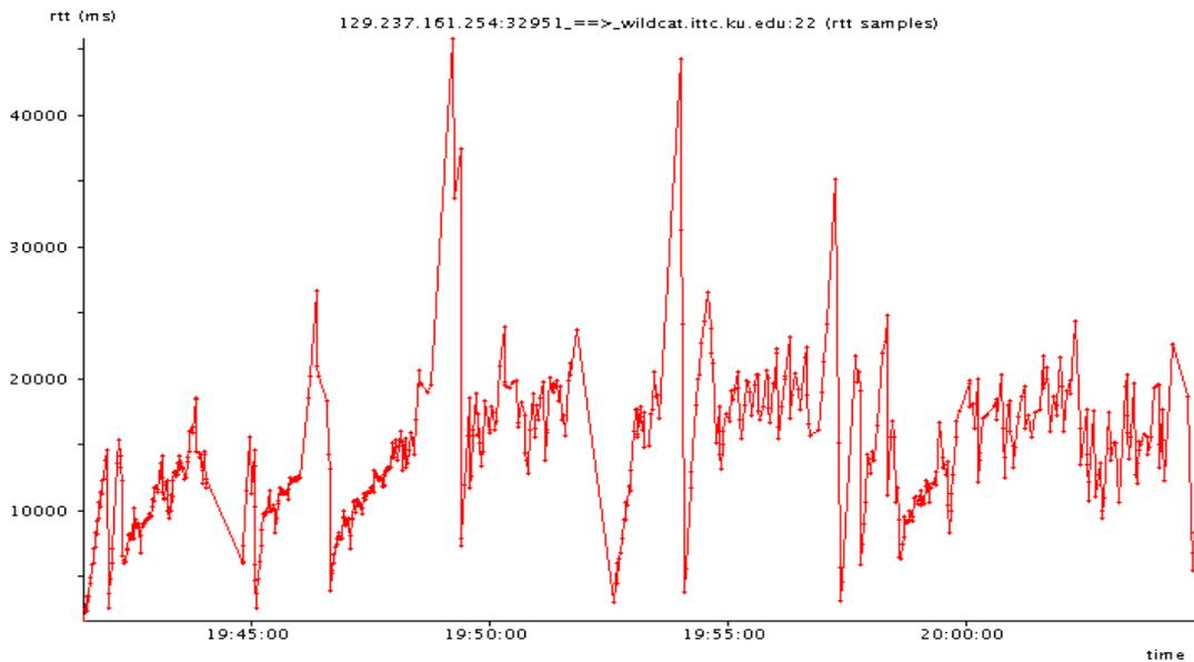
**Figure 5.22 Measured RTT during video upload**
