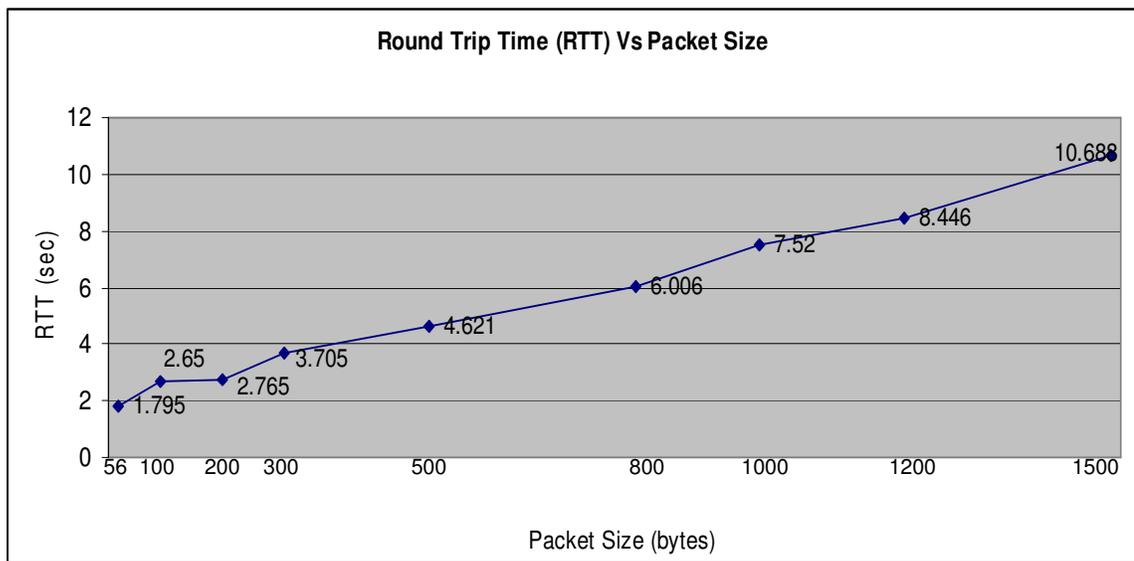
**Figure 5.5 Variation of RTT with respect to packet size**
