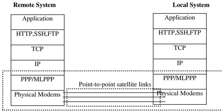
**Figure 3.2 Protocol stack of the remote and local system**
