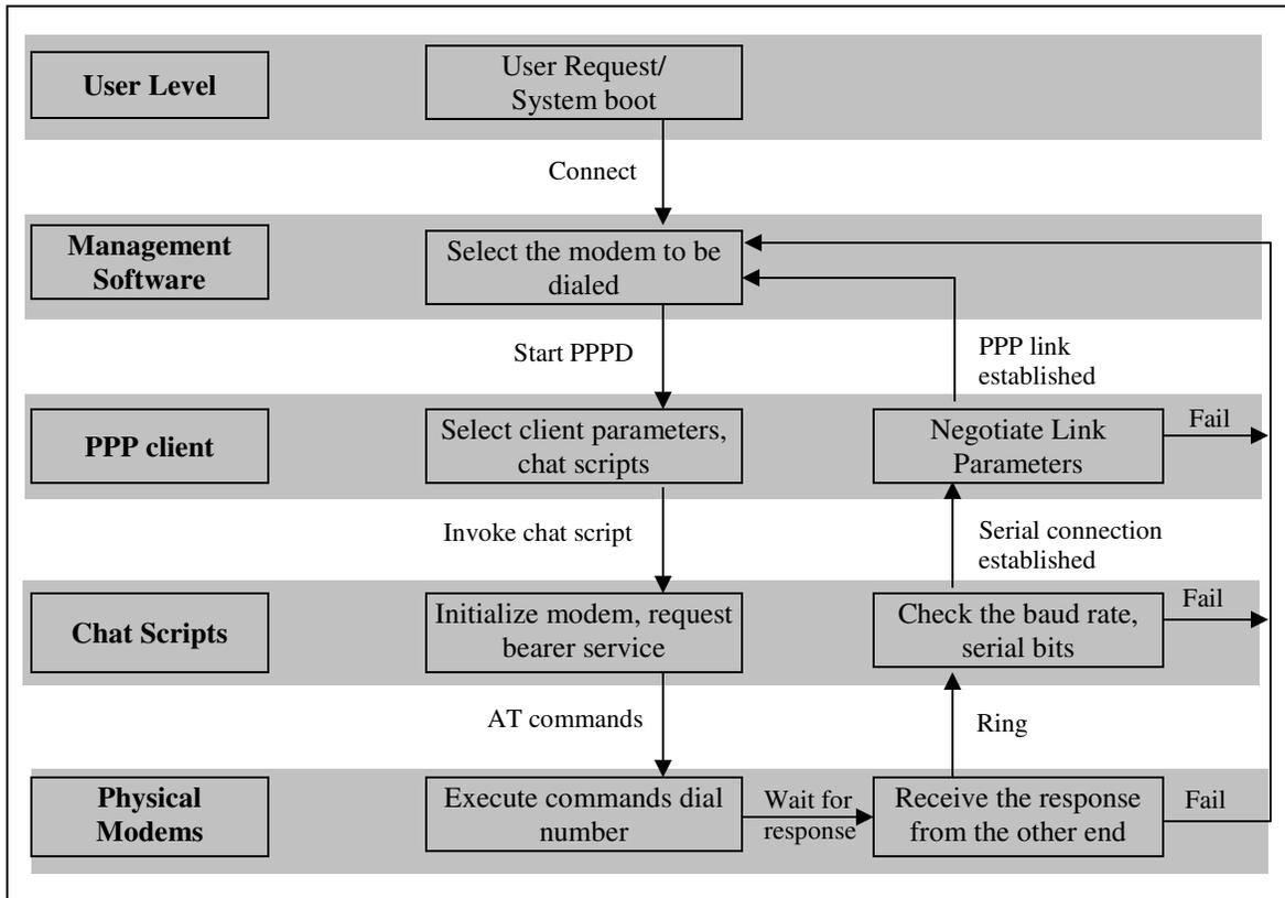
**Figure 4.3 Software flow control diagram of the remote system**
