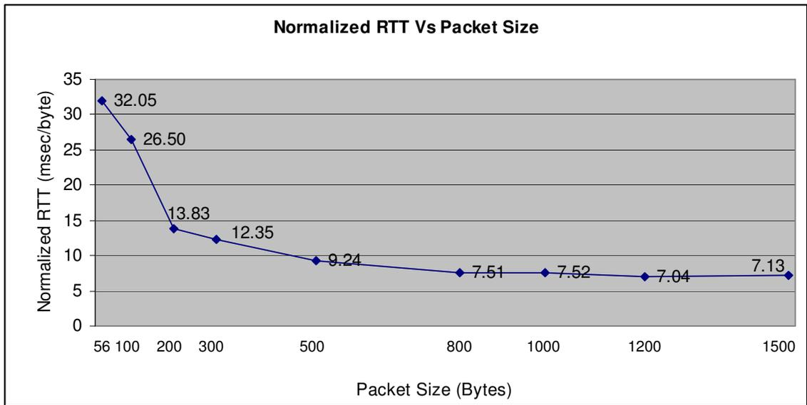
**Figure 5.6 Variation of normalized RTT with respect to packet size**
