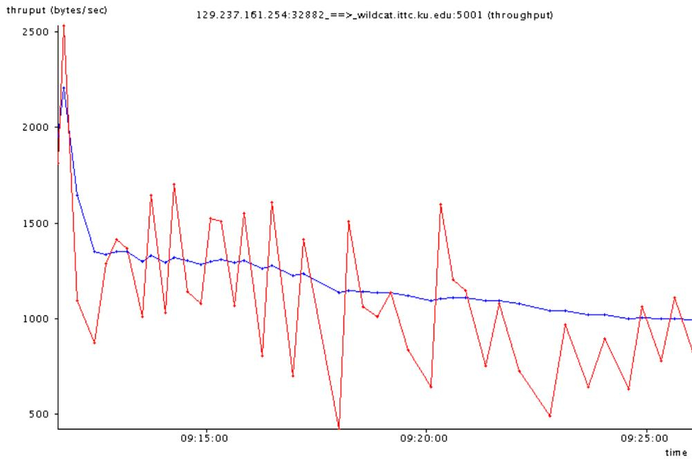
**Figure 5.27** Throughput of the TCP connection with a single call drop
