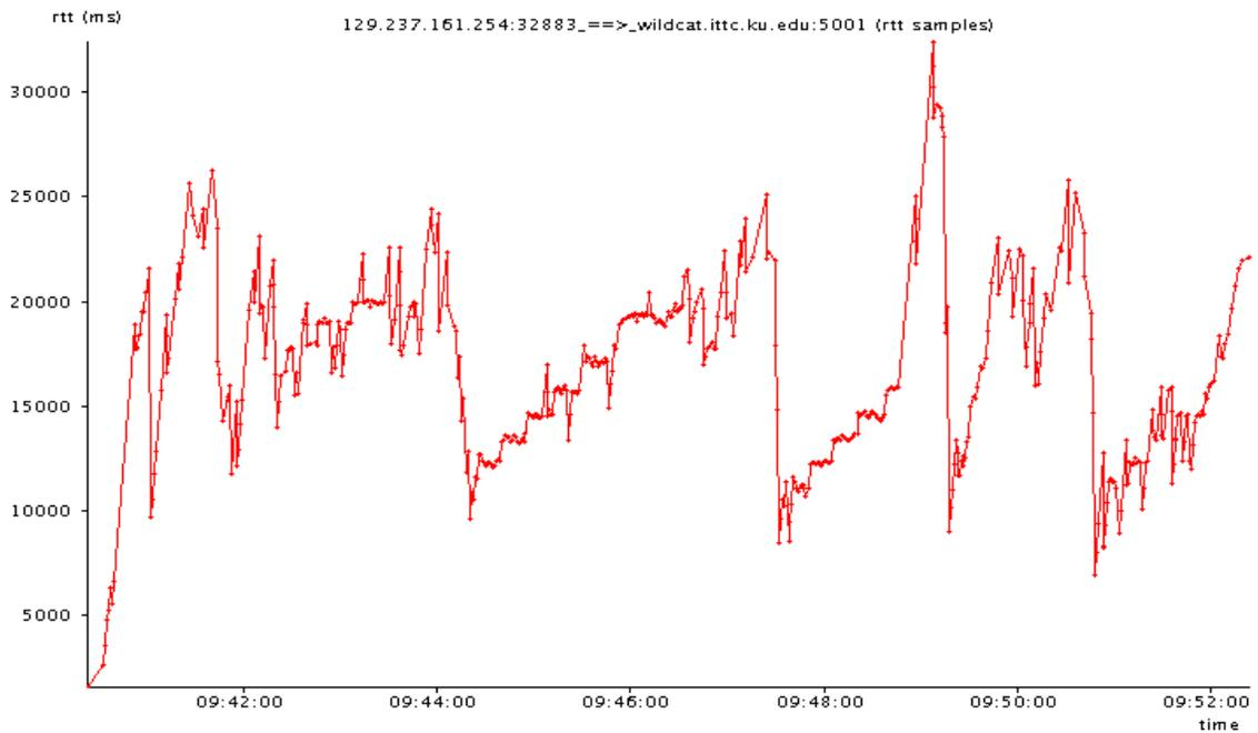
**Figure 5.15** RTT of the 4-channel Iridium communication system
