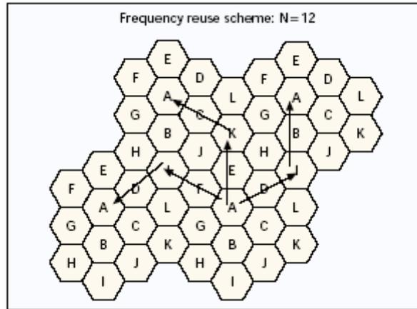
**Figure 2.7: Frequency reuse in Iridium (Source: [19])**
