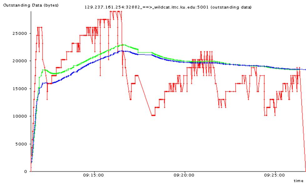
**Figure 5.25 Outstanding data window of TCP connection with a single call drop**
