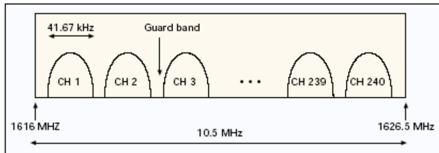
**Figure 2.5: Iridium FDMA scheme (Source: [19])**
