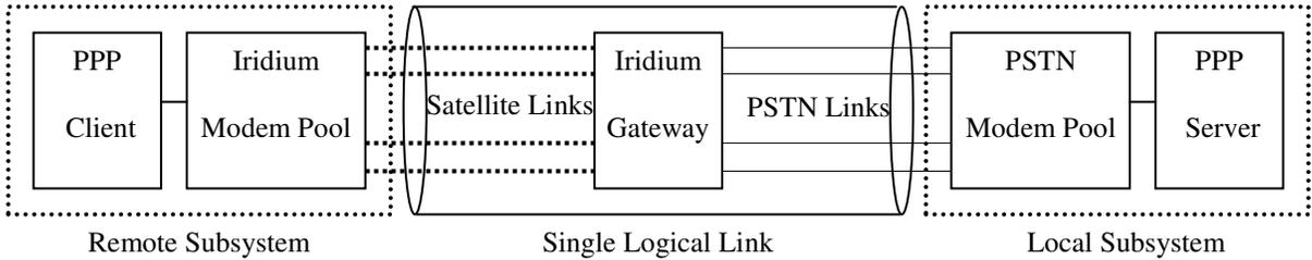
**Figure 3.1 Multi-channel data communication system**
