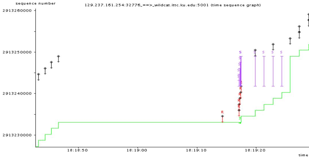
**Figure 5.29** Closer look at time sequence graph of a TCP connection with a single link termination
