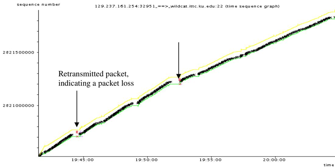
**Figure 5.19 Time sequence graph of a video upload**
