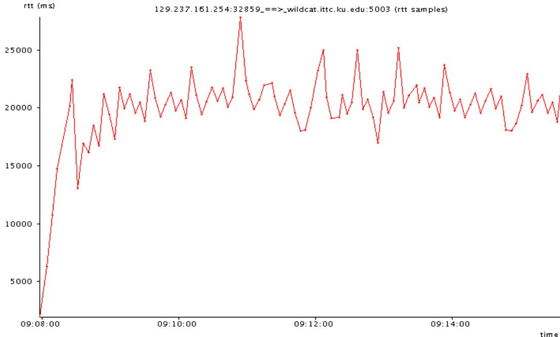
**Figure 5.13 Measured RTT of a single Iridium Link**
