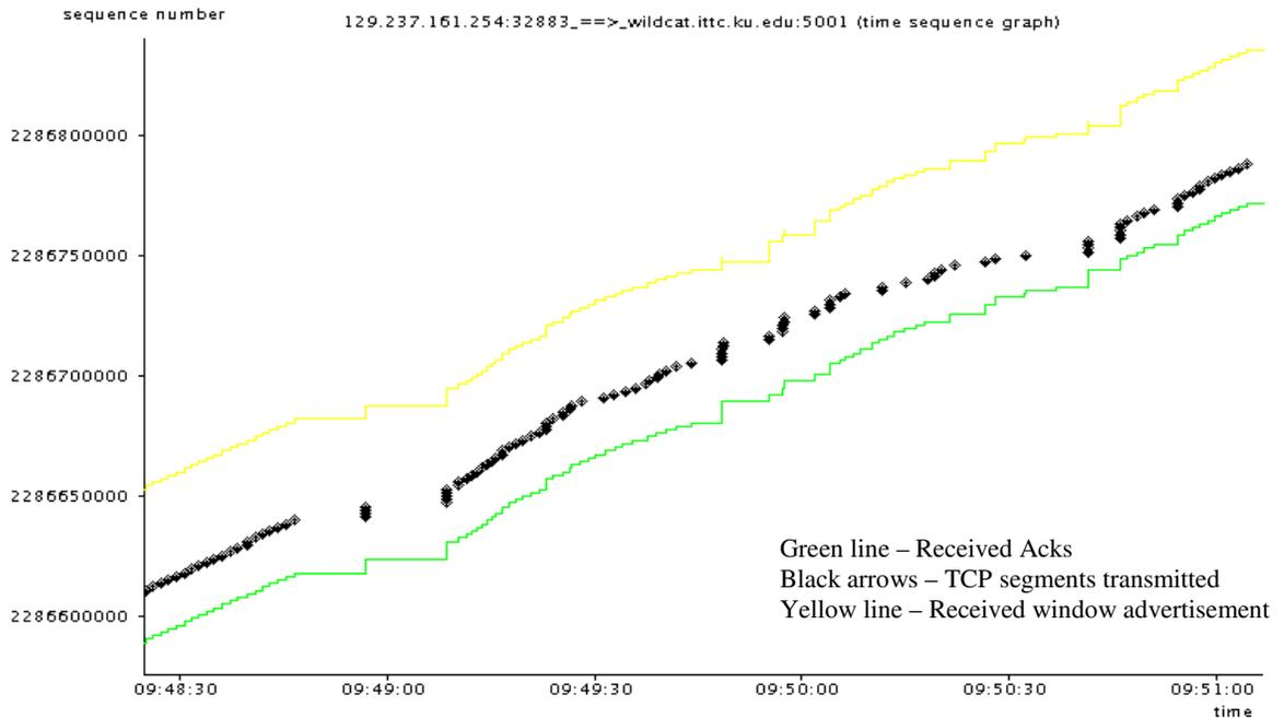
**Figure 5.17 Closer look at the time sequence graph of a 4-channel system**
