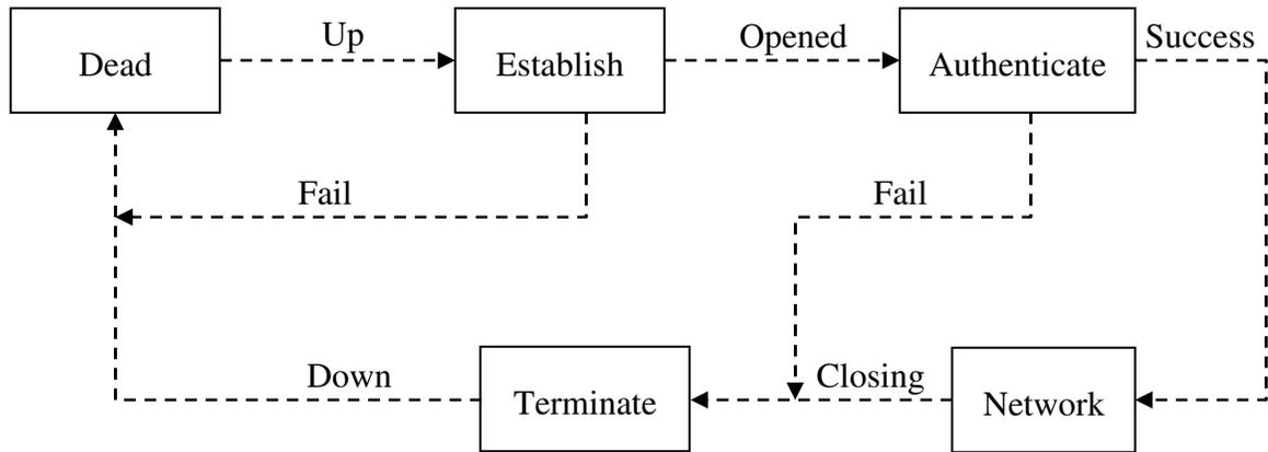
**Figure 2.14: PPP phase diagram (Source: [22])**
