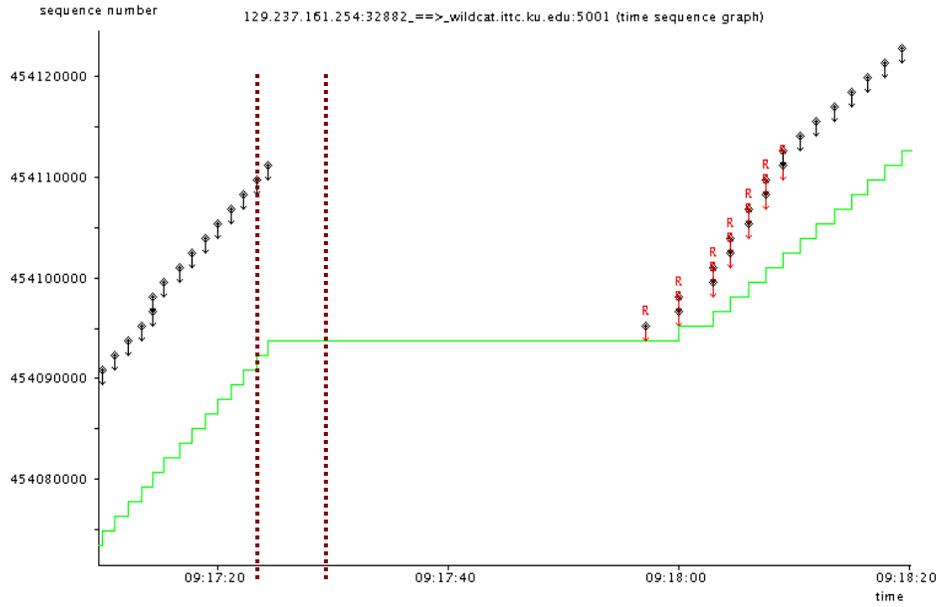
**Figure 5.26** Time sequence graph a TCP connection with a single call drop
