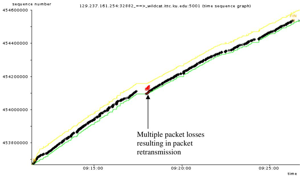
**Figure 5.24 Time sequence graph of a TCP connection with a single call drop**
