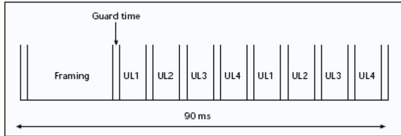
**Figure 2.8: Iridium TDMA scheme (Source: [19])**
