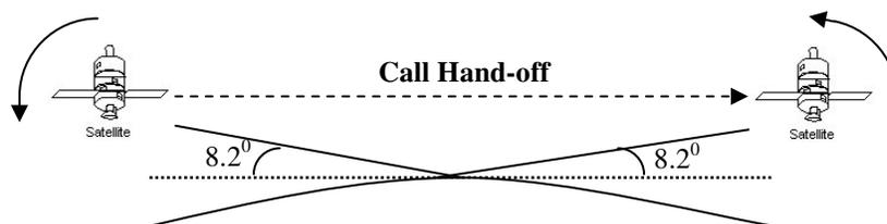
**Figure 2.3: Call hand-off between two satellites**
