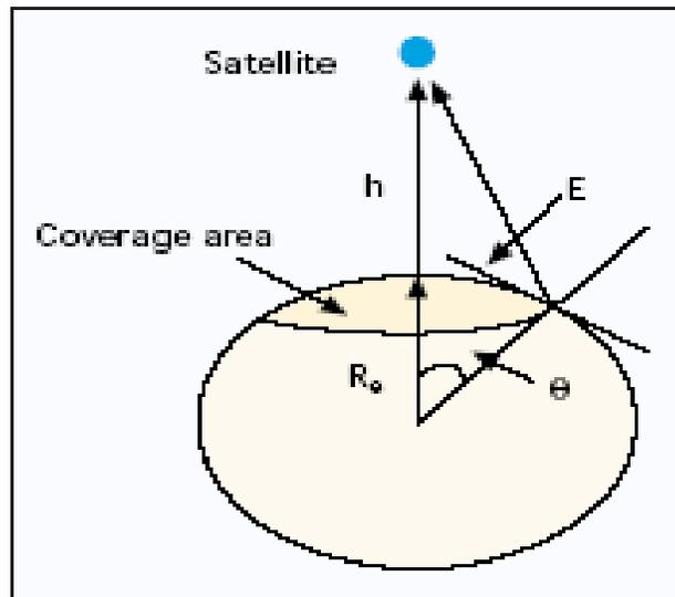
**Figure 2.4: Coverage area of a satellite (Source: [19])**
