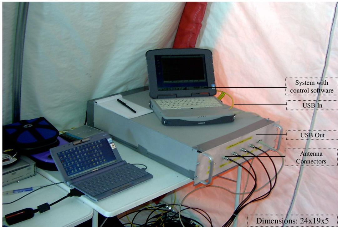
**Figure 5.1 Field implementation of multichannel Iridium communication system**
