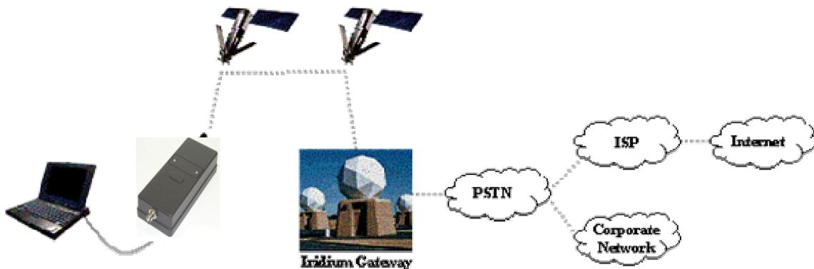
**Figure 2.10: Iridium-to-PSTN data connection (Source: [21])**
