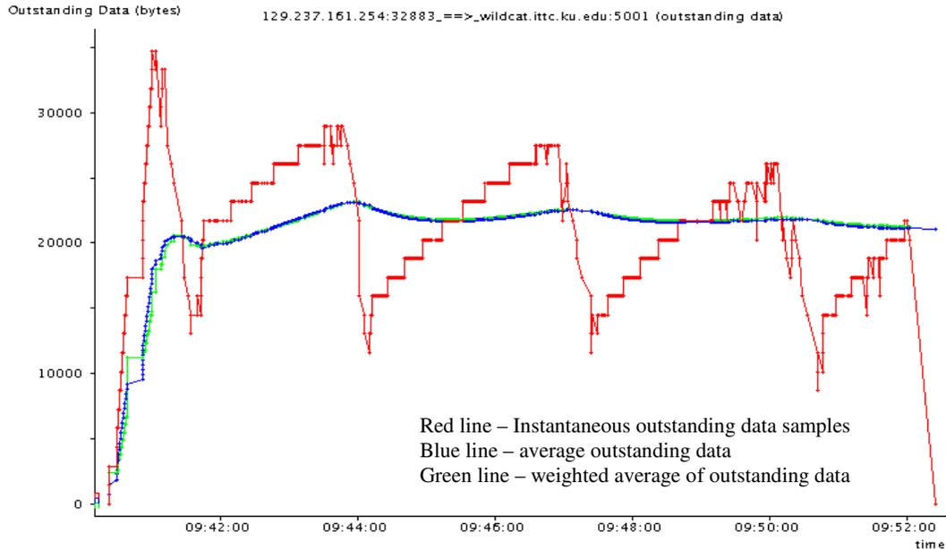
**Figure 5.18 Outstanding unacknowledged data during a TCP connection using 4-channel Iridium system**
