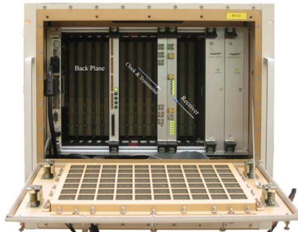
**Figure 5.3 Transmitter and Receiver compact PCI cards mounted inside Euro Cage**
