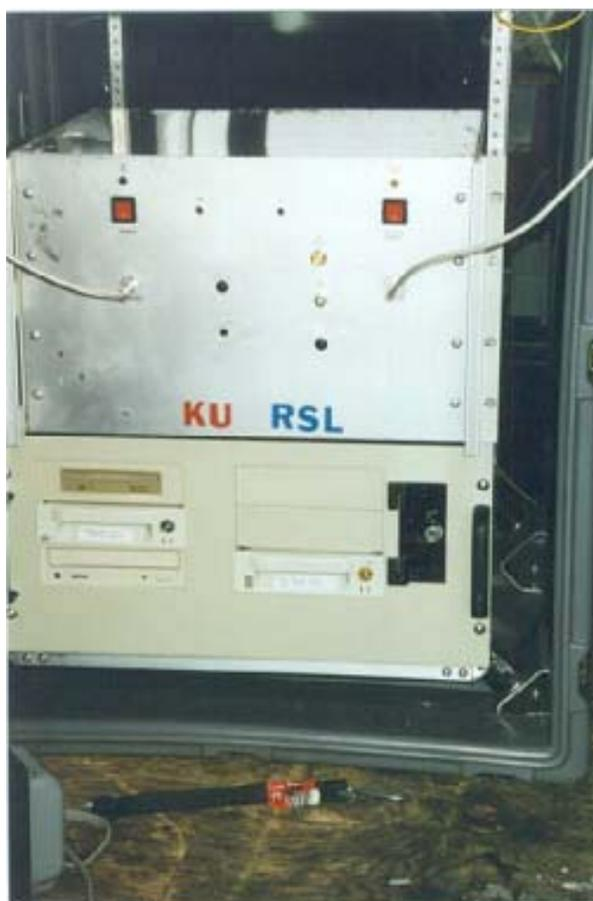
Figure 5.6. Radar system (top) and data-acquisition computer (bottom) mounted in a Hardigg box on the Trackmaster.
