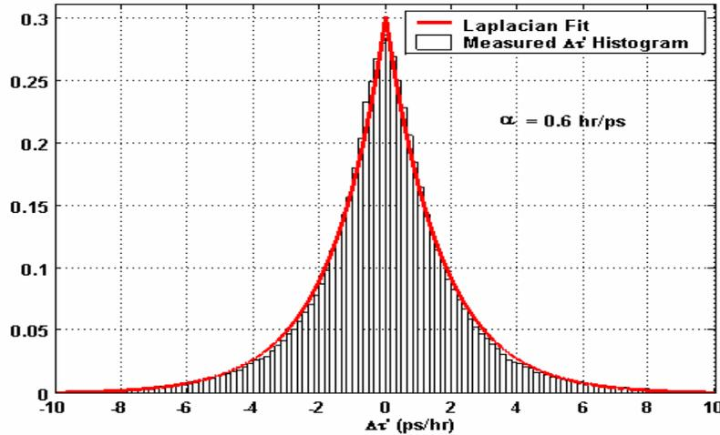
Histogram of measured  $\Delta\tau'$  data from Link 1-2 and its Laplacian fit in linear scale
