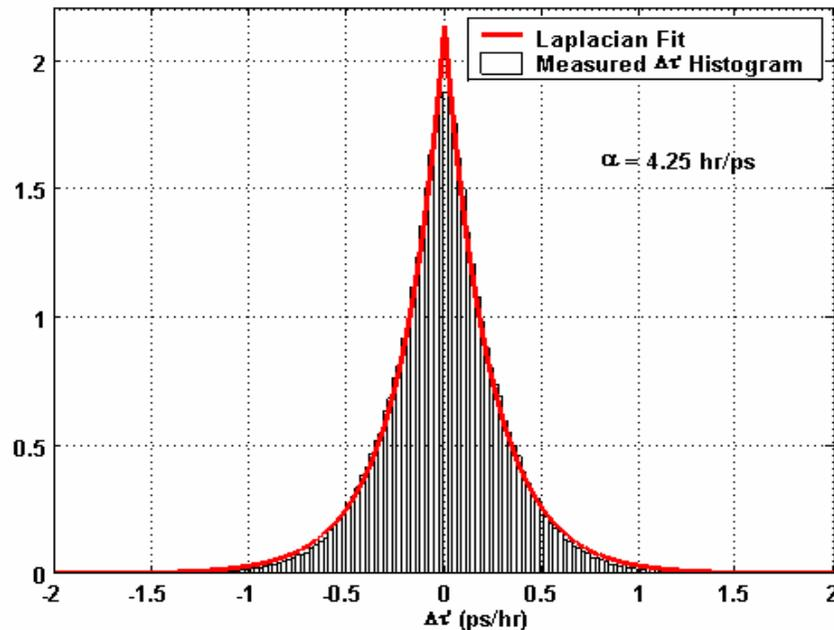
Histogram of measured  $\Delta\tau'$  data from Link 2 and its Laplacian fit in linear scale
