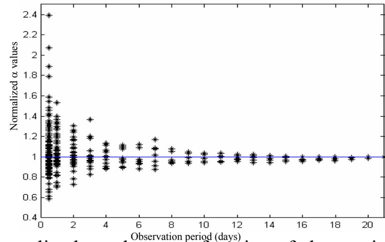
Normalized  $\alpha$  values as a function of observation period using measured data from two-span links
