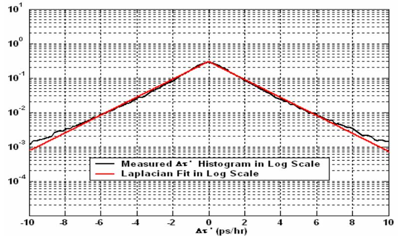
Histogram of measured  $\Delta\tau'$  data from Link 1-2 and its Laplacian fit in log scale
