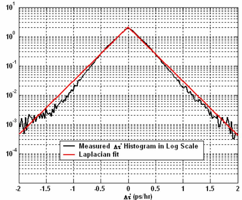
Histogram of measured  $\Delta\tau'$  data from Link 2 and its Laplacian fit in log scale
