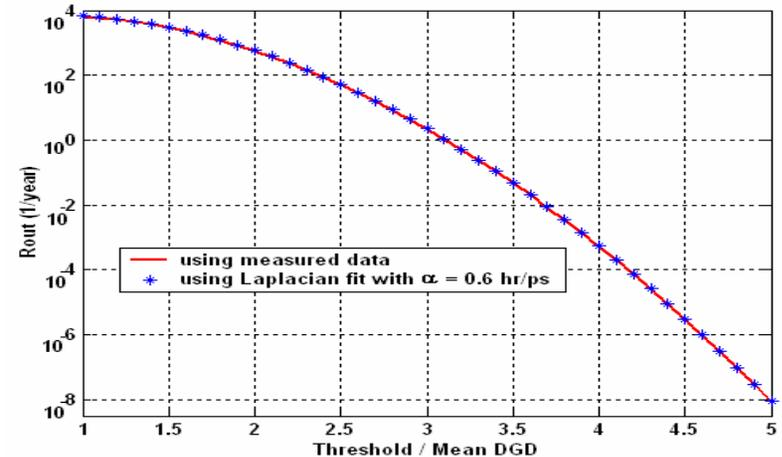
Comparison of  $R_{out}$  values on Link 1-2 calculated using original and simplified expressions
