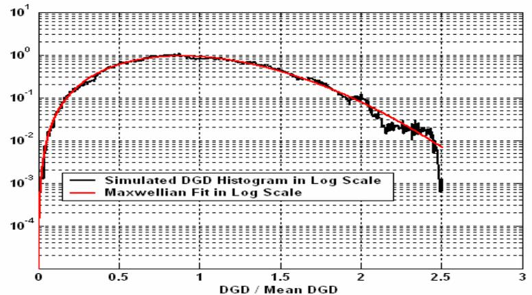
Simulated DGD time derivative histogram in linear and log scales
