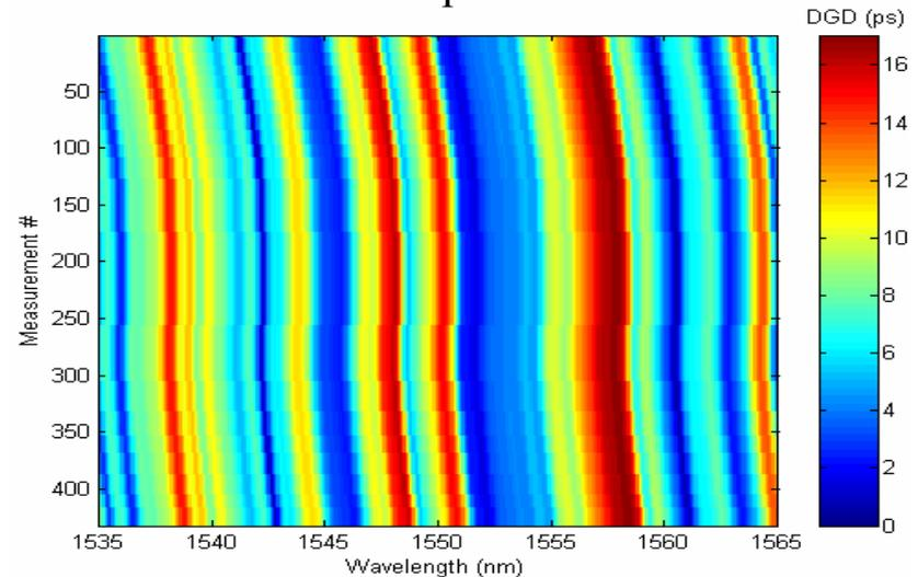
DGD vs. wavelength and time using the modeled PMD coefficient
