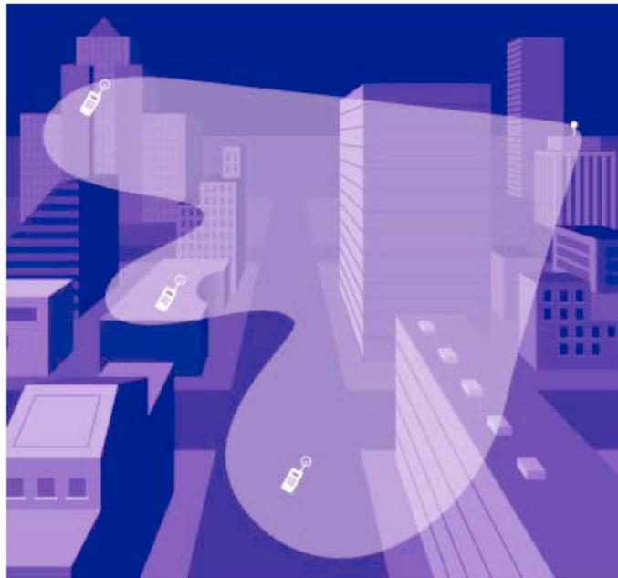
**Figure 1:6 Smart Antenna concept - Sculpted patterns to fit the topology of the sector. Minimizes transmit power, reduces interference and balances load [28]**
