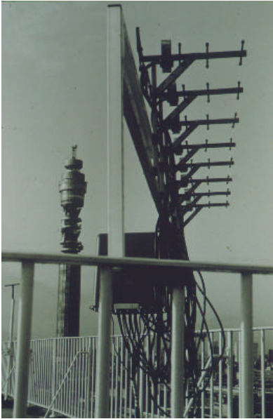
Fig. 9. Digital beamforming array used for pulse chasing experiments with UCL bistatic radar system.
