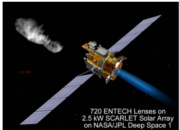
FIGURE 2. SCARLET Array on Deep Space 1 (1998-2001).
