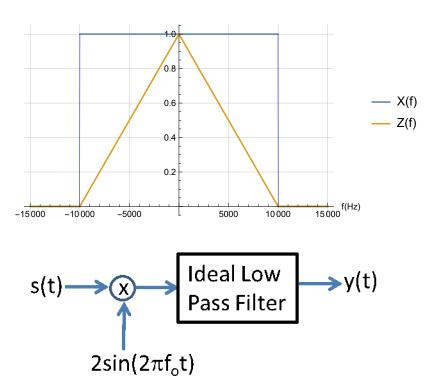
Find the output y(t) in terms of x(t) and z(t) of the system above. The bandwidth of the ILPF is 11 kHz. [Hint: use the trigonometry identities for  $\sin^2(\theta)$  and  $\cos^2(\theta)$ ]
