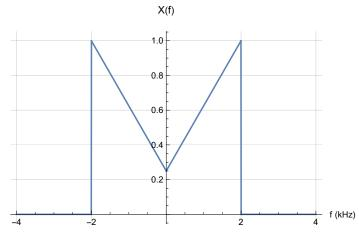
a. The signal x(t) is sampled at a rate of  $f_s$  =5000 samples/sec to create  $x_s(t)$ . Sketch the spectrum of the sampled signal  $x_s(t)$ .
