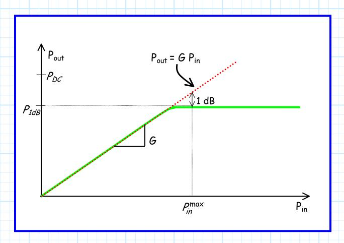
Note the equation  $P_{out}(dB) = [P_{in}(dB) + G(dB)] - 1 dB$  alone is **not sufficient** to determine the 1 dB compression point, as we have two uknowns ( $P_{in}$  and  $P_{out}$ ). We need **another** equation!
