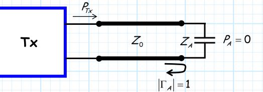
Thus, it is imperative that the impedance of an antenna have a **real** component if we wish for it to **absorb** energy, with maximum power transfer occurring when  $Z_A = Z_0$ .
