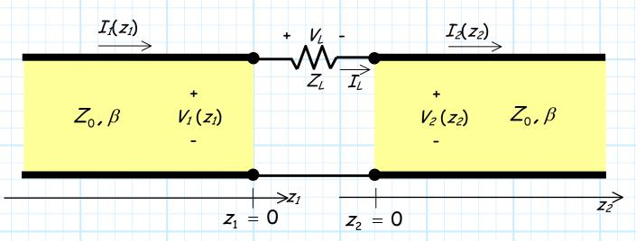
I.E., Two transmissions of **identical** characteristic impedance are connect by a **series** impedance  $Z_L$ . This second line is eventually **terminated** with a load  $Z_L = Z_0$  (i.e., the second line is **matched**).
