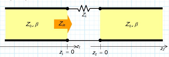
Note that since the second line is (eventually) terminated in a matched load, the input impedance at the **beginning** of the second line is simply equal to  $Z_0$ .
