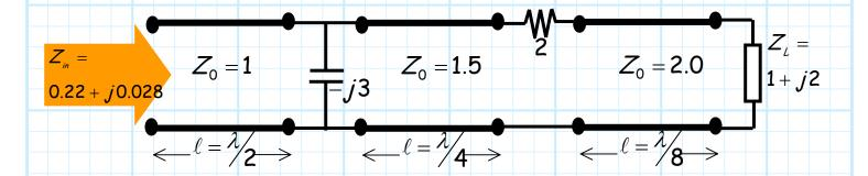
are precisely the **same**! They have **exactly** the same impedance, and thus they "behave" precisely the **same** way in any circuit (but **only** at frequency  $\omega_0$ !).
