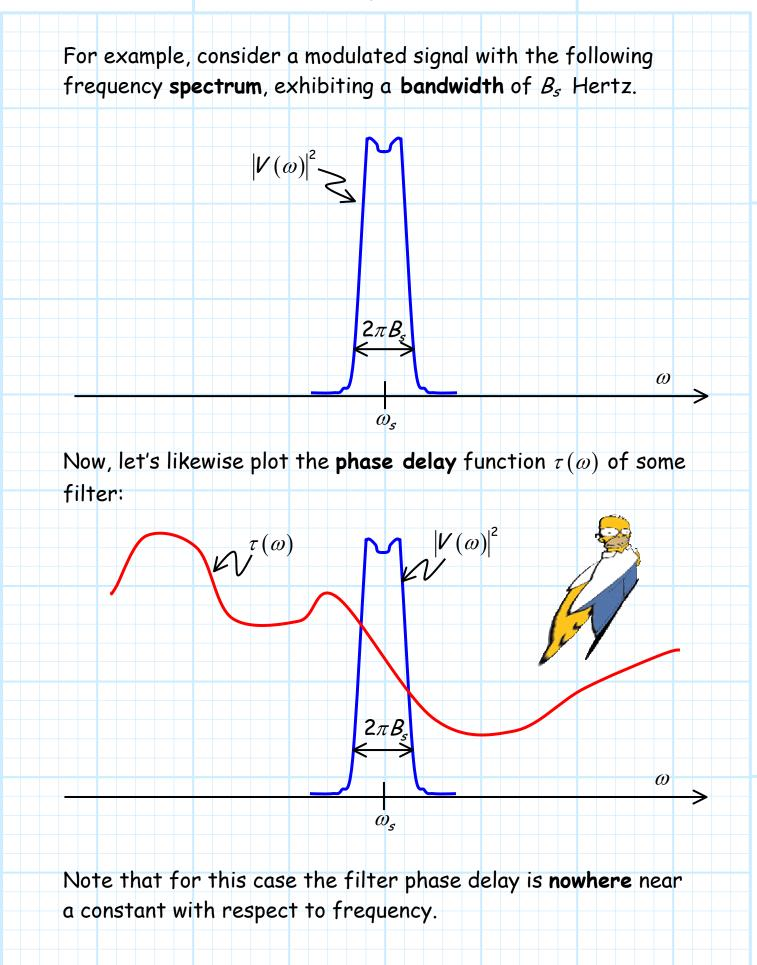
However, this fact alone does **not** necessarily mean that our signal would suffer from **dispersion** if it passed through this filter. Indeed, the signal in this case **would** be distorted, but **only** because the phase delay  $\tau(\omega)$  changes significantly across the **bandwidth**  $B_s$  of the signal.
