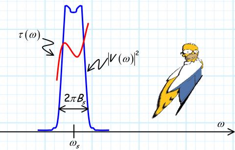
Thus, a narrowband filter (e.g., IF filter) must exhibit a near constant phase delay  $\tau(\omega)$  in order to avoid distortion due to signal dispersion!
