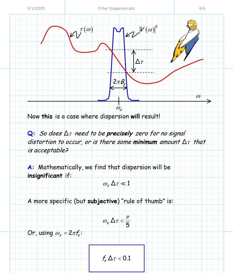
**Generally** speaking, we find for **wideband** filters—where filter bandwidth *B* is much greater than the signal bandwidth (i.e.,  $B \gg B_s$ )—the above criteria is **easily** satisfied. In other words, signal dispersion is **not** typically a problem for wide band filters (e.g., preselector filters).
