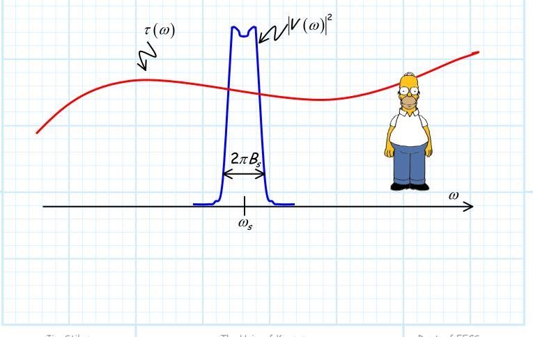
Conversely, a **narrowband** filter—where filter bandwidth *B* is approximately **equal** to the signal bandwidth (i.e.,  $B_s \approx B$ )—can (if we're not careful!) exhibit a phase delay which likewise changes **significantly** over **filter** bandwidth *B*. This means of course that it **also** changes significantly over the **signal** bandwidth  $B_s$ !
