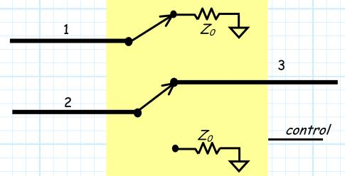
These ideal switches are called matched, or absorptive switches, as ports 1 and 2 remain matched, even when not connected.
