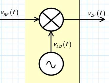
Generally, the signal delivered to the Local Oscillator **port** is a **large**, pure tone generated by a device called—a **Local Oscillator**!
