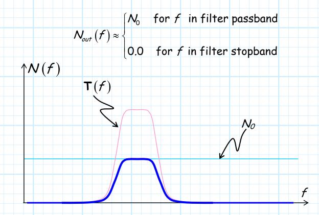
Now, if the filter has a **passband** that extends from frequency  $f_1$  to frequency  $f_2$  (i.e., bandwidth  $B = f_2 - f_1$ ), the **total power** of the noise at the **load** is:
