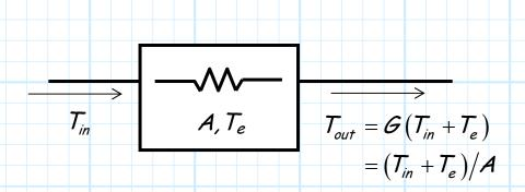
Thus, we find that the **output** noise temperature of a **passive** device is:
