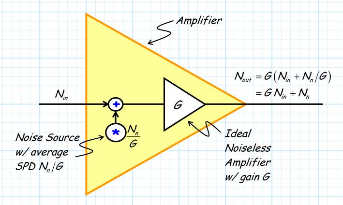
Note here that the noise source near the **input** of the amplifier has an average spectral power density of  $N_n/G$ .
