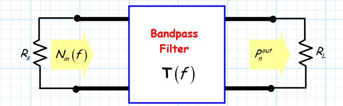
We'll consider the resistor on the **left** to be **source** of thermal noise, with average spectral power density:
