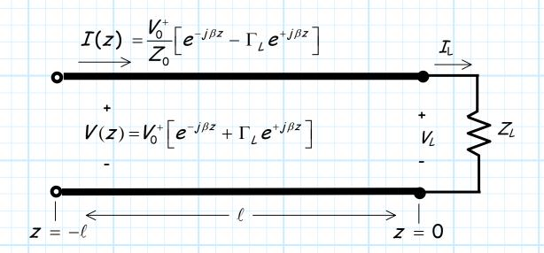
The result is that electromagnetic energy flows along the transmission line at a given rate (i.e., power).
