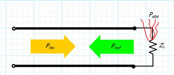
Note that if  $|\Gamma_L|^2 = 1$ , then  $P_{inc} = P_{ref}$ , and therefore **no power** is absorbed by the **load**.
