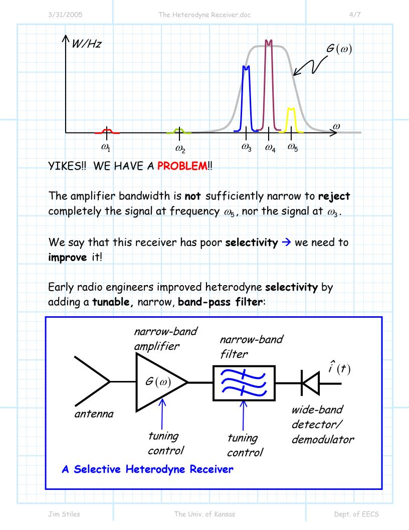
Therefore, if we tune **both** the amplifier and filter to frequency  $\omega_4$ , we might get:
