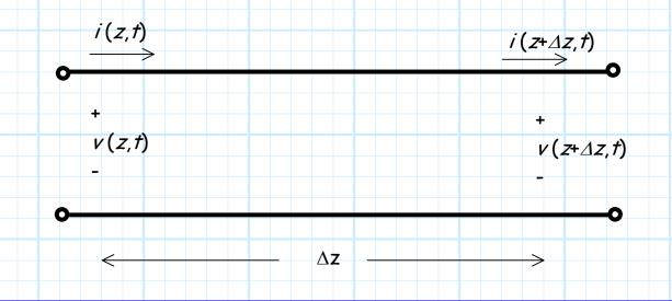
Q: Huh ?! Current i and voltage v are a function of **position** z ?? Shouldn't  $i(z,t) = i(z + \Delta z,t)$  and  $v(z,t) = v(z + \Delta z,t)$  ?
