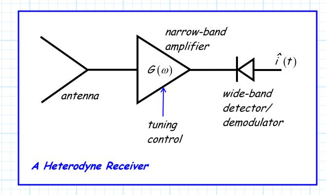
The **desired** radio signal was selected by **tuning** a narrow-band amplifier!
