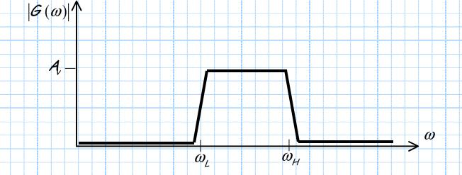
One result of having a **finite bandwidth** is that the amplifier impulse response is **not** an impulse function!
