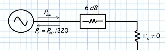
The reason that the return loss improves by 12 dB (as opposed to 6 dB) is that reflected power is attenuated **twice**—once as it travels toward the load, and again after it is reflected from it. Note from the standpoint of the source, the load is much **better matched**. As a result, the effect of **pulling** is reduced.
