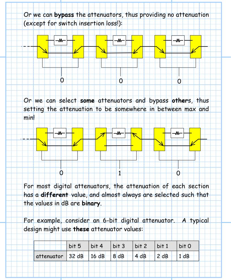
We note therefore, that by selecting the proper switches, we can select **any** attenuation between 0 dB and 63 dB, in **steps** of 1 dB.
