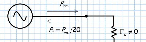
Say we now add a 6 dB pad between the source and the load we find that the return loss has **improved** to 25 dB!
