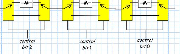
Theoretically, we can construct a digital attenuator with as many sections as we wish. However, because of switch insertion loss, digital attenuators typically use no more than 8 to 10 bits (i.e., 8 to 10 sections).
