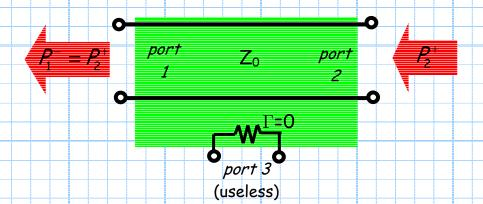
But, this is **not** true for a circulator. If power is incident on port 2, then **no power** will exit port 1!
