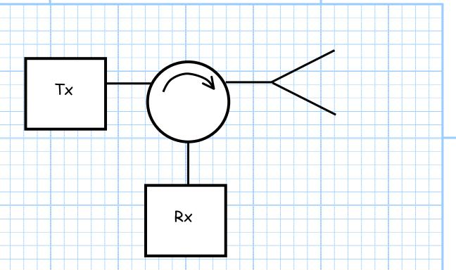
It is particularly important to keep the transmitter power from getting to the receiver. To accomplish this, the antenna must be matched to the transmission line. Do you see why?
