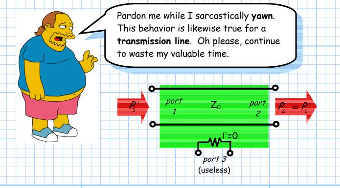
True! But a transmission line, being a **reciprocal** device, will likewise have the property that power **incident** on **port** 2 will completely **exit port** 1  $(P_1^- = P_2^+)$ :
