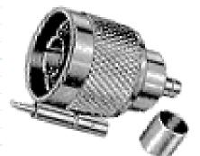
N The **original** microwave connector. Good performance (up to 18GHz), and moderate cost, but large (about 2 cm in diameter)! However, can handle greater **power** than SMA.
