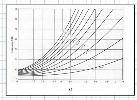
While the normalized attenuation chart for a **Chebychev** with **0.5 dB** of passband ripple is:
