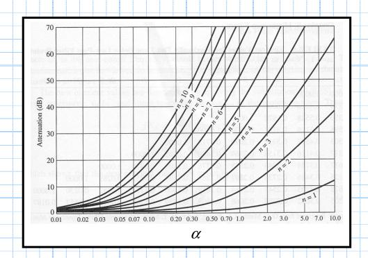
And the normalized attenuation chart for a Chebychev with 3.0 dB of passband ripple is:
