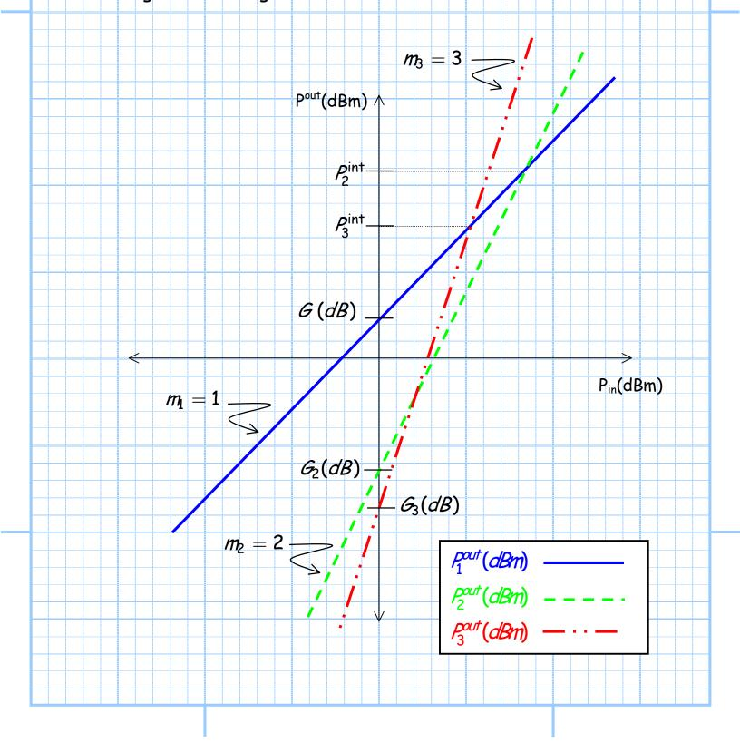
Note that for  $P_{in}(dBm) < 0 dBm$  (the left side of the plot), the second and third-order products are small compared to the fundamental (first-order) signal.
