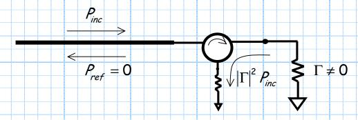
There is **no power** reflected back to the source! Instead, power reflected by the load is **absorbed** by the isolator.
