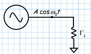
Unfortunately, the **impedance** of this load can affect the operating **frequency** of the oscillator! As  $\Gamma_L$  changes, so can the frequency  $\omega_0$  (e.g.,  $\omega_0(\Gamma_L)$ ).
