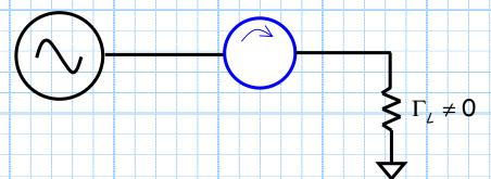
Recall that an amplifier typically has very large reverse isolation, so that we can use it to isolate the oscillator as well:
