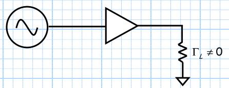
In either case, the oscillator "thinks" it is delivering its power to a matched load. The frequency of the oscillator will therefore be its nominal (i.e., matched load) value, even though the load may be poorly matched.
