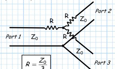
For this design, the ports are matched! However, the resistors make the device lossy:
