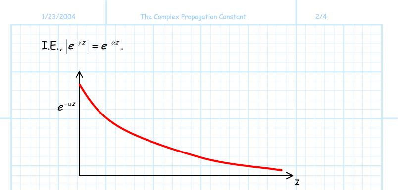
Therefore,  $\alpha$  expresses the **attenuation** of the signal due to the loss in the transmission line.
