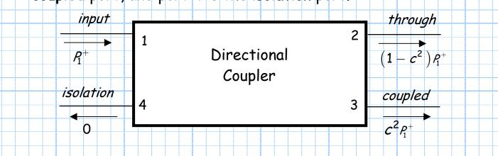
Note however, that any of the coupler ports can be an input, with a different through, coupled and isolation port for each case.
