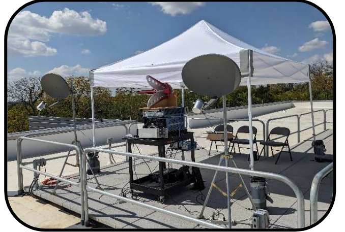
Fig. 1. Open air experimental setup with two transmitters (left/right dish antennas) and one collocated radar receiver (middle quad-ridge horn). The displaced communications receiver at 175m distance is not shown.
